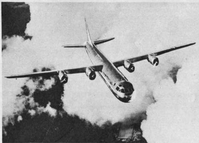
Pilot's enclosure forms slight bulge on the liner's long rounded nose as graceful Davis wing suspends its heavy, awkward-looking fuselage.
